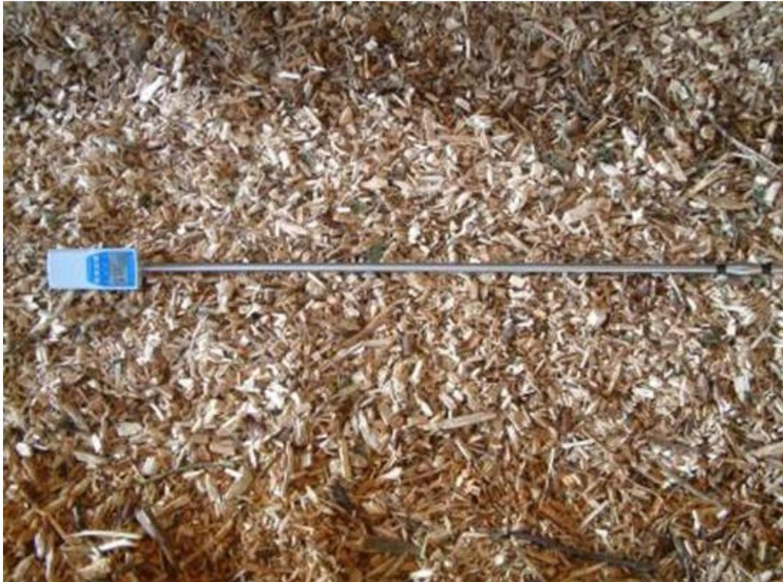
Biomass moisture content should be measured precisely by the moisture meter.
