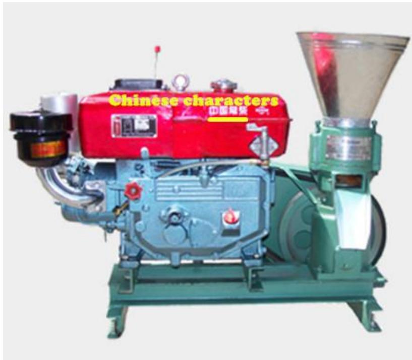
Diesel pellet mill from [makeyourownpellets.com](http://makeyourownpellets.com)
