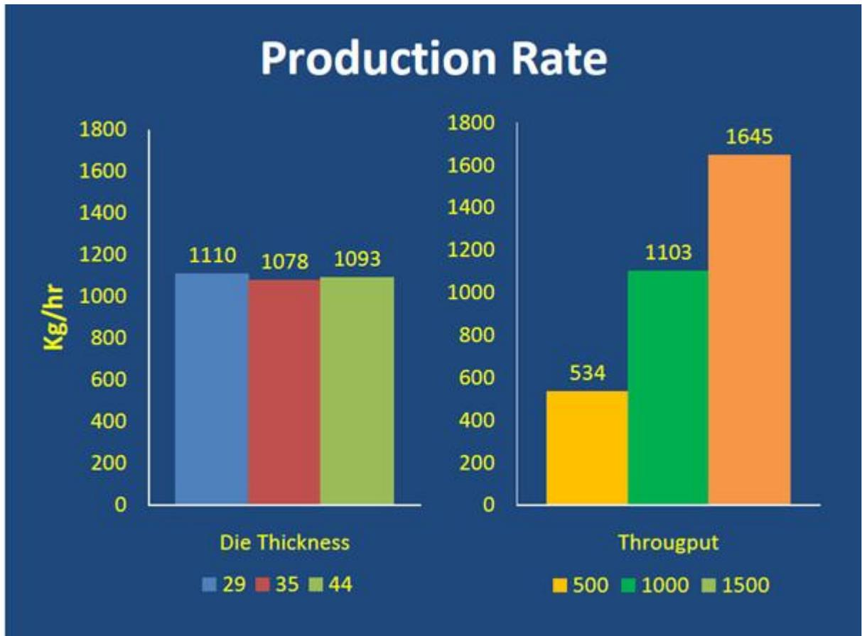
Negative effect of pellet die thickness to the pellet production rate.
